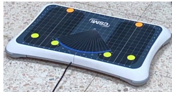
Figure 3. Humac platform with adhesive dots for the same foot position to be maintained for the same participant during the reassessment
