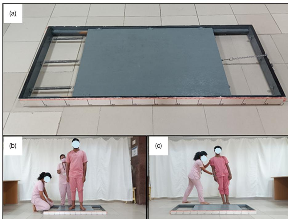
Figure 1. (a) moving platform, (b) testing of reactive lateral stepping using the moving platform, (c) testing of reactive lateral stepping using the BESTest
