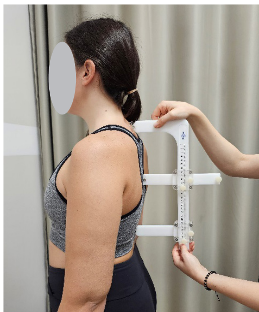
Figure 2. Illustration of the D'Oswaldo arcometer application for sagittal plane measurement (demonstrated by an adult model for ethical compliance)
